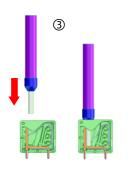
Insert the conductor with ferrule or the solid conductor into the round input.
