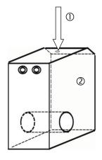
➤ If water sprays from the vent hole ① of the measuring chamber ②, reduce the amount of inlet water via the manually operated shutoff valve. It should take 2 to 6 seconds to fill the measuring chamber!
